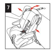
With weakest hand at belt path, tilt and push the child restraint forward and back and side to side. If the seat belts do not loosen, your child restraint should be secure.
